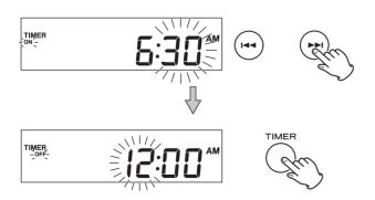
"TIMER" and "OFF" indiactors appear on the display and the "hour" value starts flashing.
